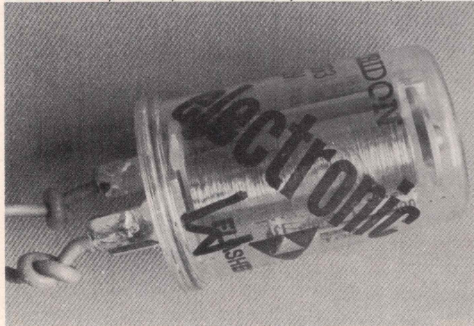
A 6 volt Volkswagen blinker can is all you need to run-in your stock motors by the motor-zapping method.
