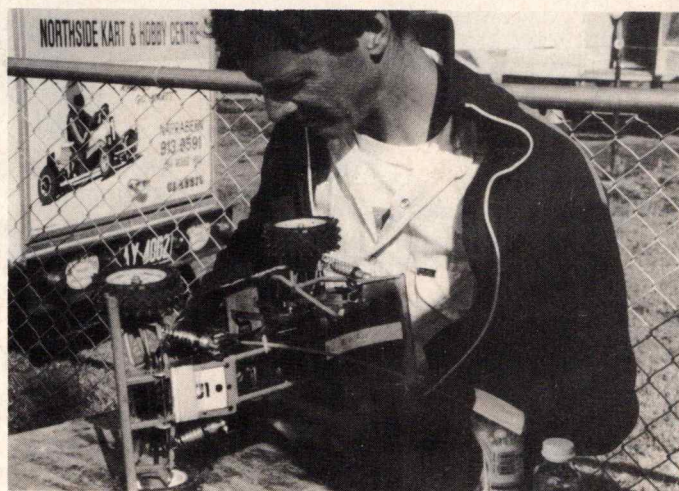
Bob Inglis of Bankstown with his Zerda. Has Supershot rims all round, MRC tyres, Option House shocks and inboard USR stock motor. Made the A Final. MG pic.
